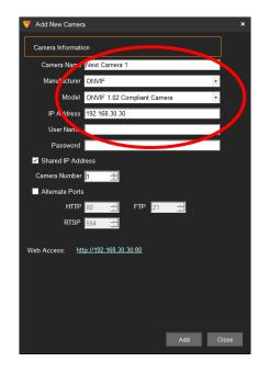
Video Insight configures multi-video devices as "Shared IP" devices. Thus, the "Shared IP Address" must be selected as well as selecting the appropriate video input (camera number). Leave the "Alternate Ports" element unchecked. Then click the "Add" button to add the video stream to the system database.
